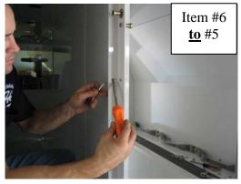
Loosely attach **Doorframe** to **Center divider** using #10 x 3/8" flat head machine screws and nylock nuts
